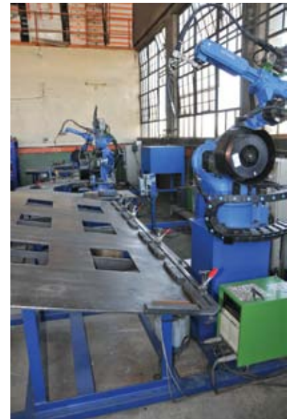
World Power Products has four Motoman robots of various sizes carrying out robotic welding operations
