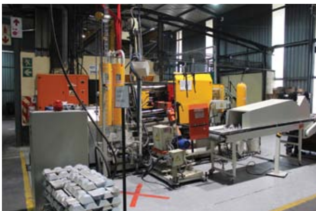
The project involved the purchase of a 160 ton hot chamber HPDC machine from Taiwanese manufacturer Producer CO Ltd
