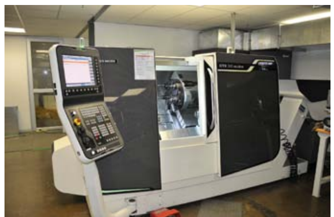
On the turning side there is a DMG MORI CTX 310 ecoline
