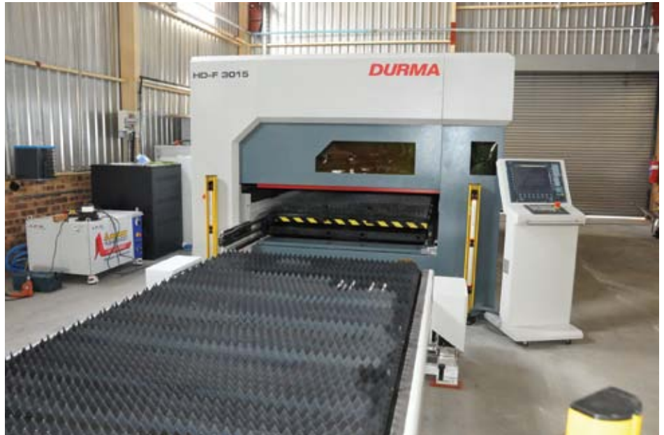
The new Durma HD-F 3015 4kW fibre laser with a cutting length of 3000mm and cutting width of 1500mm was installed in April 2016
