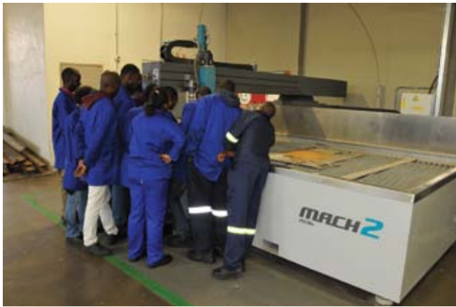
Students being trained on the Flow mach 2031b waterjet
