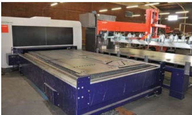
The new Bystronic Bysprint 4020 6kw fiber laser comes with automatic loading and unloading
