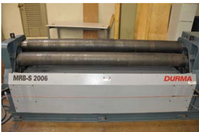
Included in the sheetmetal department is a Durma MRB-S 2006 three roll bending machine
