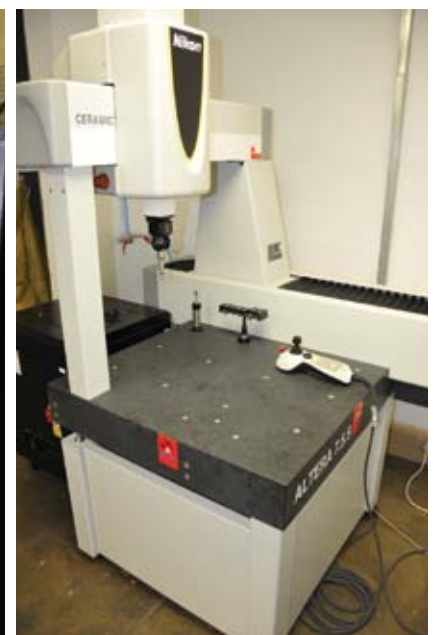
Just installed is a Nikon Altera 7.5.5 coordinate measuring machine, supplied by WD Hearn Machine Tools
