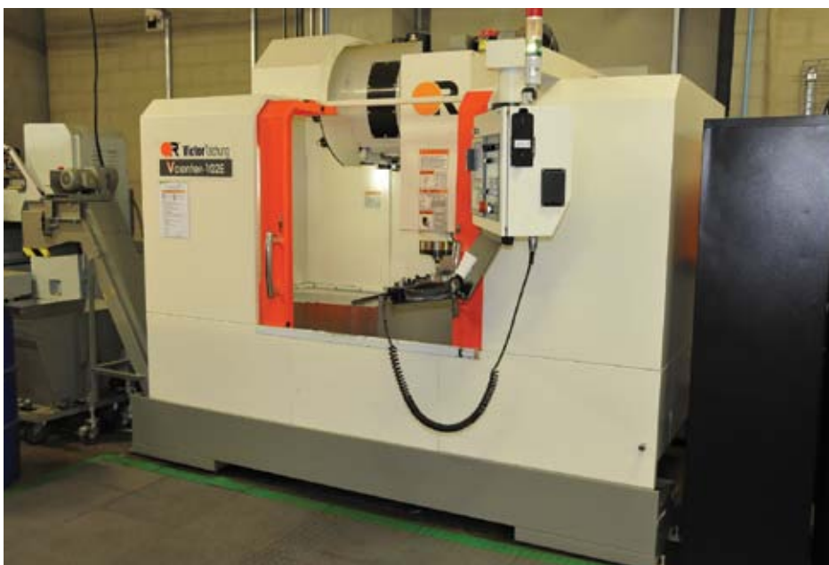
The Resolution Circle have also installed a Victor Vcenter-102E CNC vertical machining center
