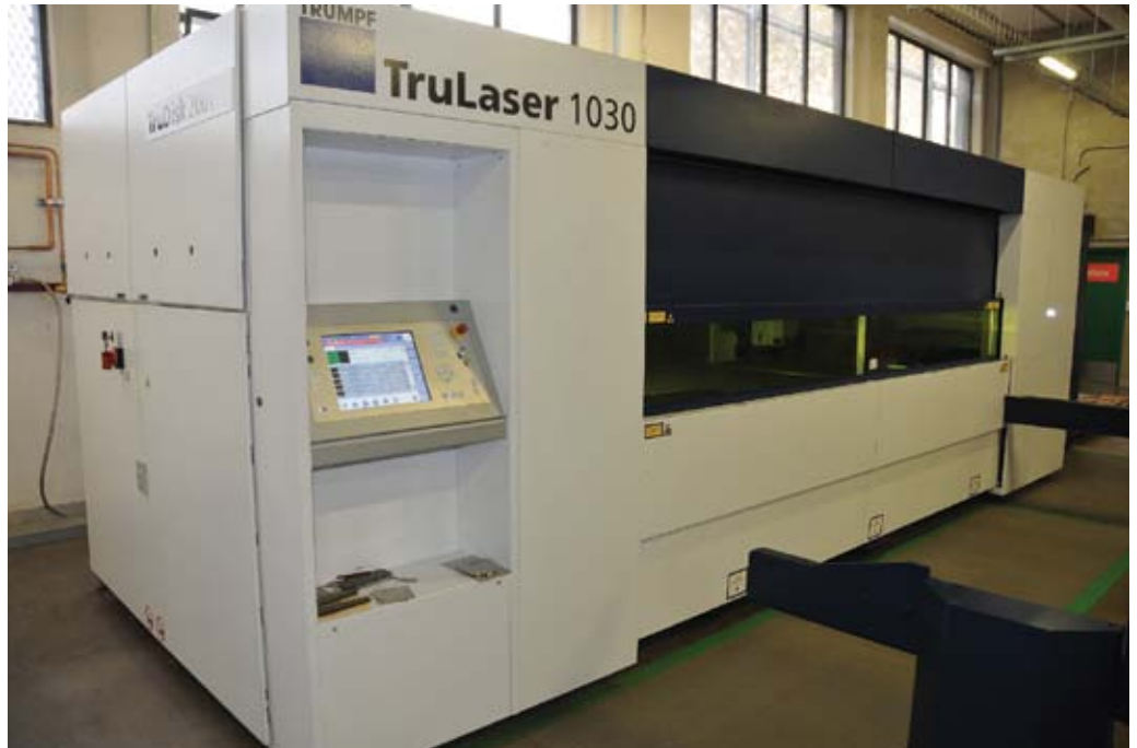
The laser installed at Resolution Circle is a Trumpf TruLaser 1030 fiber laser. The machine was installed by Retecon Machine Tools
