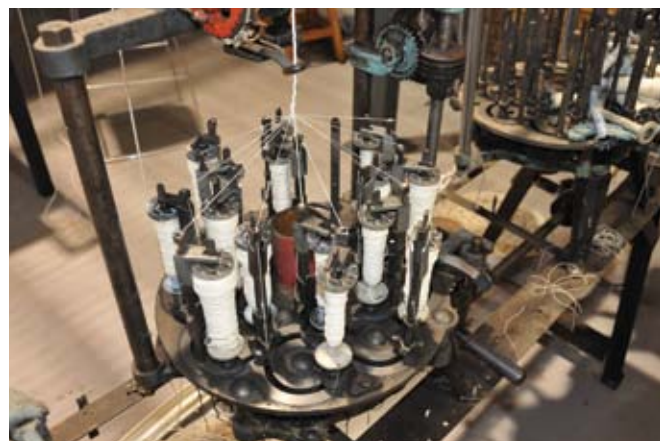
Enviro Lamps believes in manufacturing its own moulds and components that make up that product, including weaving the wicks for the oil lamps
