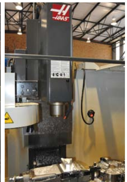
The first CNC machine that Enviro Lamps purchased was a Haas TM-2 Toolroom mill
