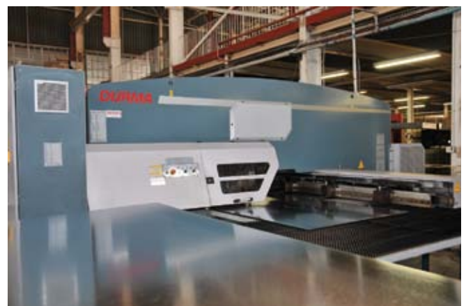
Edge Line Engineering has also recently installed a Durma turret punch press
