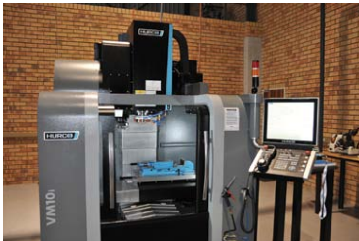
Another recent purchase was a Hurco VM10i vertical machining centre that was supplied by Hurco South Africa
