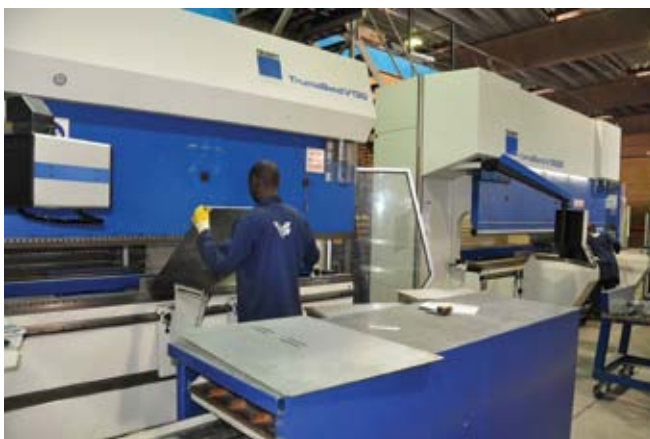
World Power Products has over 30 press brakes, the bulk of them being Trumpfs, and the largest a 320 ton Trumpf
