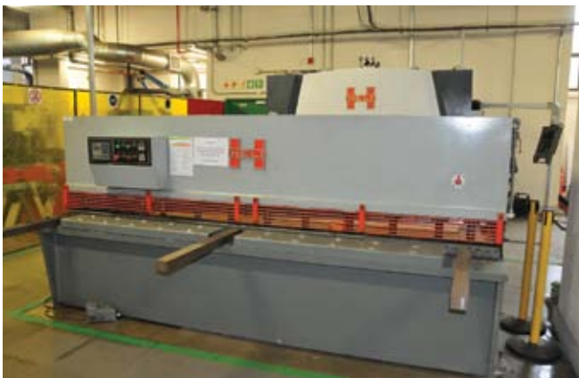
In the bending department there is a Heli 125 ton 3 metre press brake and a Heli 6mm by 3200mm guillotine
