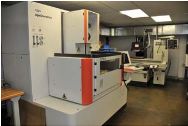
Retecon Machine Tools have also installed an AgieCharmilles CUT 20 P. In the background is the Chevallier FSG-1632ADIII-1640ADIII high-precision 3-axes automatic surface grinder
