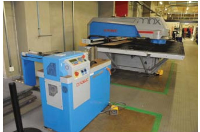
Two Euromac machines have been installed by CML Machine Tools. The first machine, a Euromac MBX 1250/30-2250mm, is an autoindex CNC punching machine that uses the Euromac multitool system, and the second machine is a Euromac Digibend 400 bending machine with a 40 ton force
